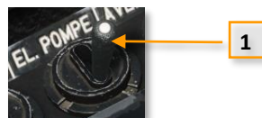
Figure 3-25 Electro-Pump Switch in Right Console
