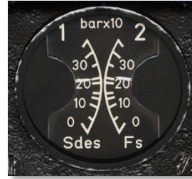
Figure 3-32 Dual Hydraulic Pressure Gauge in Main Panel
