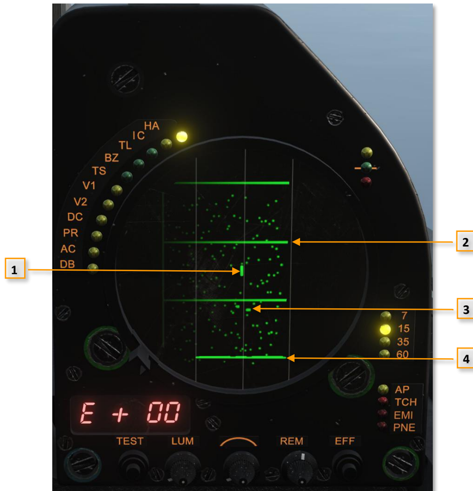
Figure 3-113 Radar Before Lock-on
