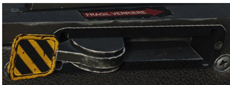
Figure 3-61 Canopy Embrittle Control in Left Wall
