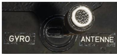
Figure 3-96 Antenna-Gyro Switch in Left Console
