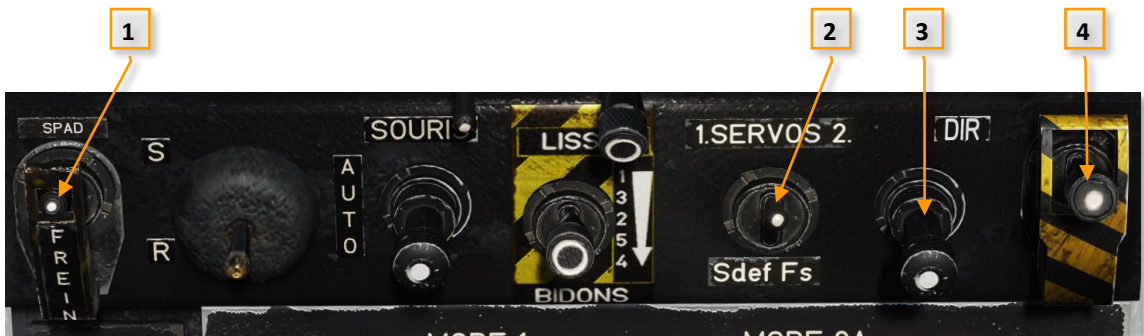
Figure 3-29 Hydraulic System Controls in Main Panel
