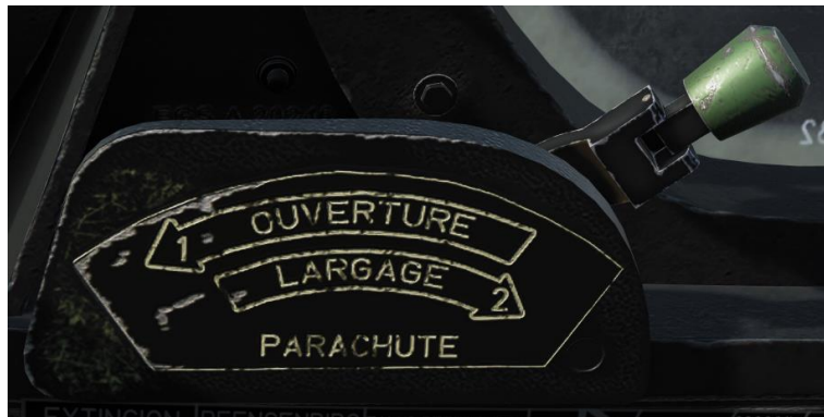
Figure 3-49 Brake Chute Control Lever In Left Wall
