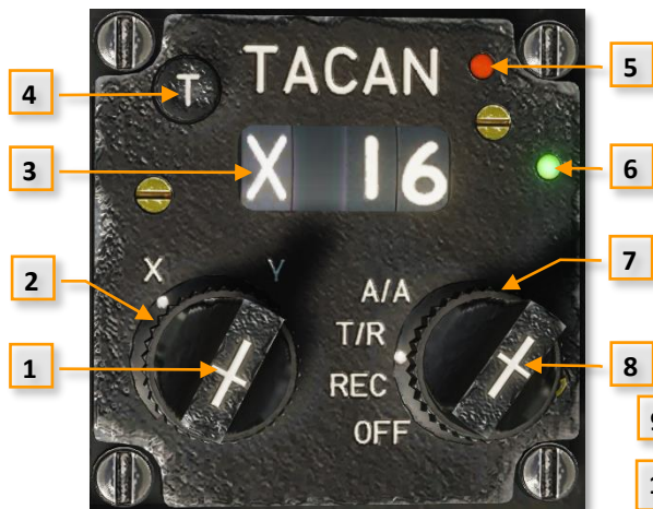
Figure 3-90 TACAN Control Unit in Right Console
