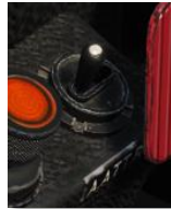
Figure 3-69 Landing Light Control in Left Console
