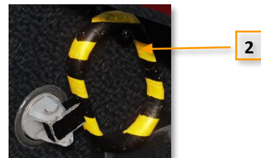
Figure 3-26 Emergency U/C Handle in Right Front Panel
