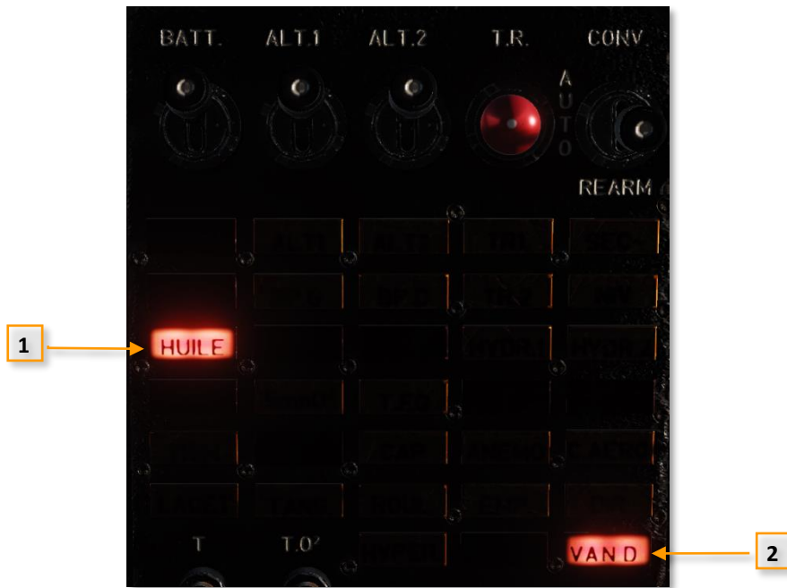
Figure 3-23 Failure Warning Panel
