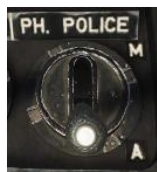
Figure 3-71 Search Light Control in Right Console
