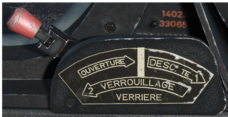
Figure 3-60 Canopy Lock Control in Right Wall
