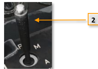
Figure 3-19 Firing Fuel Dipper Switch in Right Console
