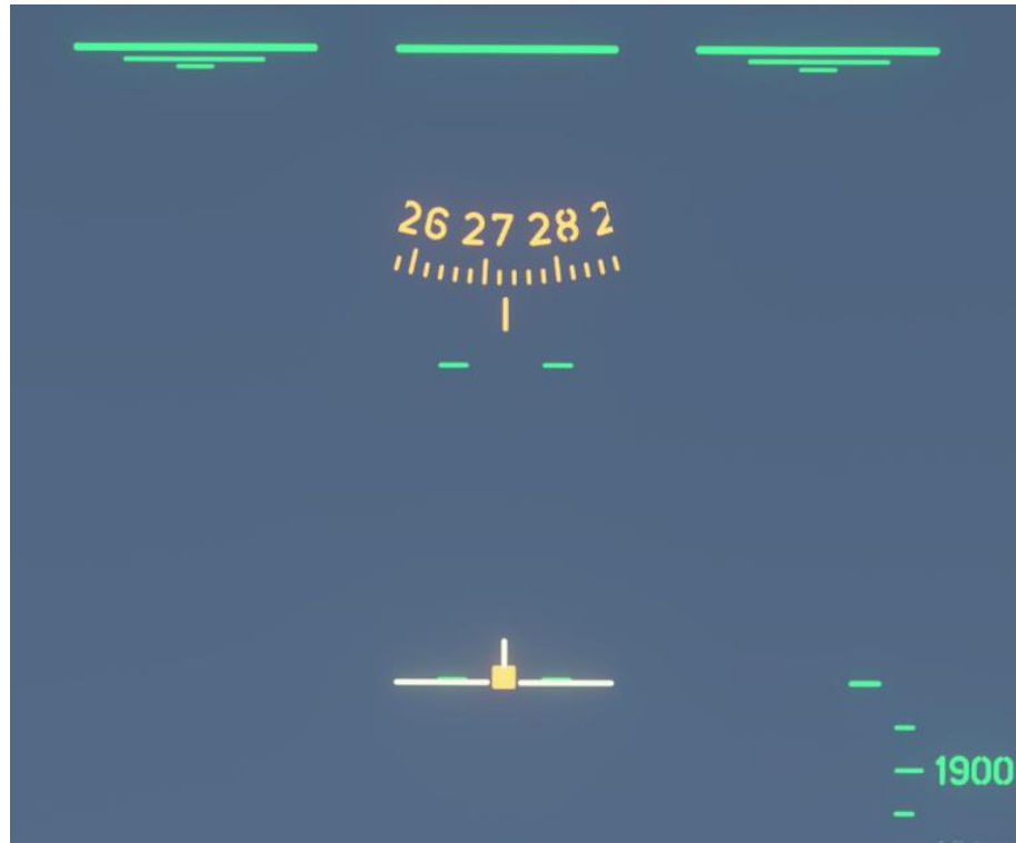
Figure 4-2 Sight approach mode display without airbrakes
