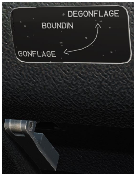
Figure 3-76 Canopy Seal Valve Control Lever in Right Wall
