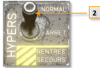
Figure 3-28 High-lift Device Selector Switch in Left Console
