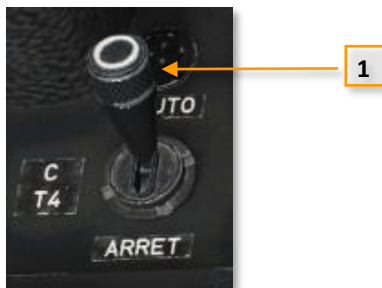
Figure 3-18 JPT Emergency Regulation Switch in Left Console
